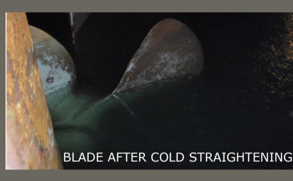
BLADE AFTER COLD STRAIGHTENING.
